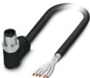
Sensor/Actuator cable, 5-position, PE-X halogen-free, black, shielded, Plug angled M12 SPEEDCON, A-coded, on free cable end, Cable length: 2 m, For railway applications
