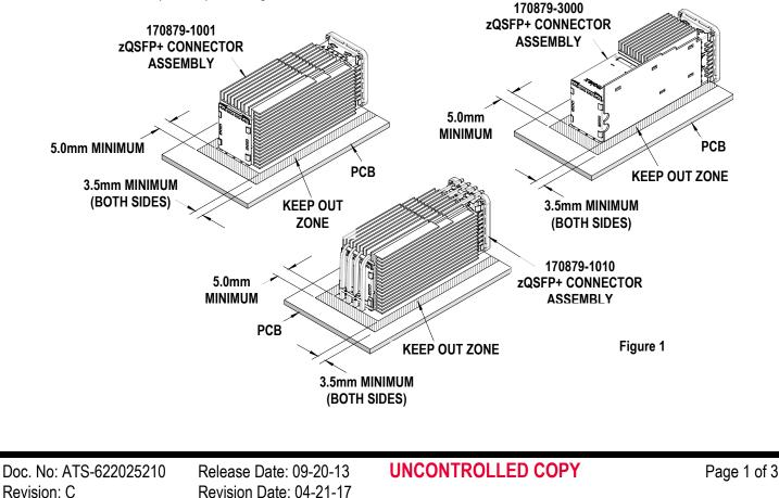
zQSFP+ Multi-Port Connector Tooling
