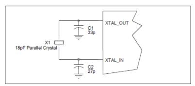
FIGURE 2. CRYSTAL INPUT INTERFACE
