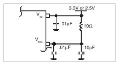
FIGURE 1. POWER SUPPLY FILTERING
