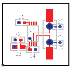
FIGURE 5B. 844031I-01 PC BOARD LAYOUT EXAMPLE
