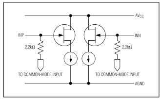
Figure 2. Simplified Analog Input Architecture
