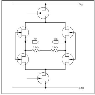
Figure 5. Simplified LVDS Output Architecture
