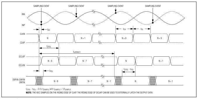
Figure 4. System and Output Timing Diagram
