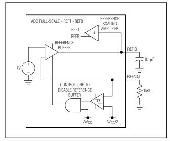
Figure 3. Simplified Reference Architecture
