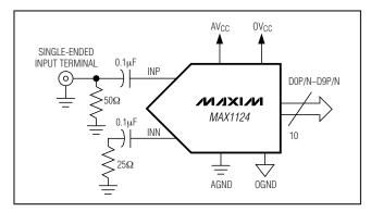
Figure 9. Single-Ended AC-Coupled Analog Input Configuration
