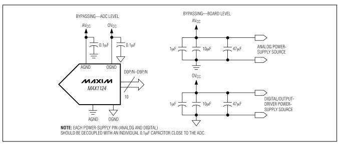
Figure 10. Grounding, Bypassing, and Decoupling Recommendations for the MAX1124
