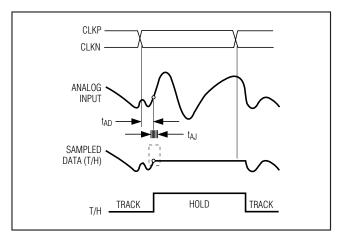
Figure 11. Aperture Jitter/Delay Specifications
