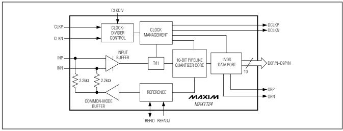
Figure 1. MAX1124 Block Diagram
