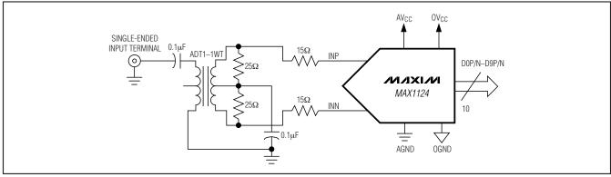
Figure 8. Transformer-Coupled Analog Input Configuration with Secondary-Side Termination
