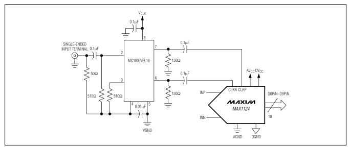
Figure 7. Differential, AC-Coupled, PECL-Compatible Clock Input Configuration
