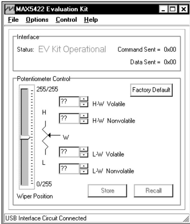
Figure 1. MAX5422 Evaluation Kit Software Main Window
