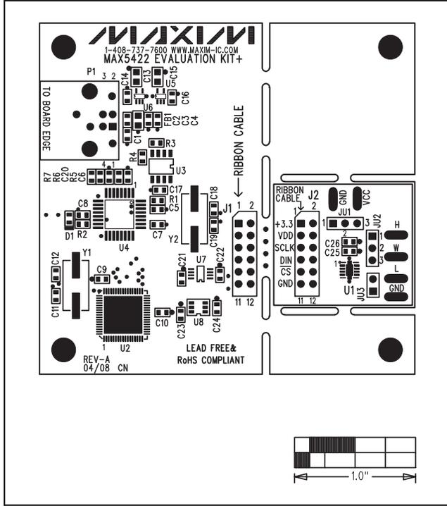
Figure 5. MAX5422 EV Kit Component Placement Guide—Component Side
