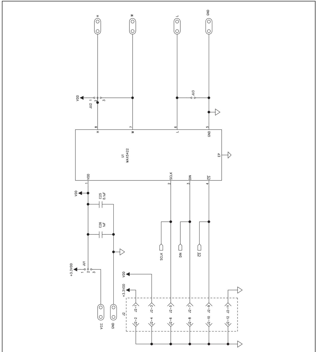
Figure 4a. MAX5422 EV Kit Schematic (Sheet 1 of 2)
