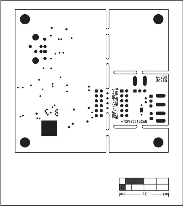
Figure 8. MAX5422 EV Kit Component Placement Guide—Solder Side
